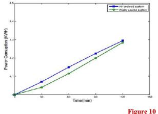
Graph between energy consumption with Air cooled and Water cooled Condenser of Refrigerator Vs Time
