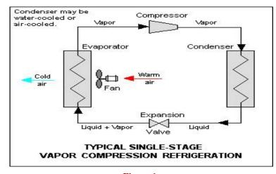
Vapor compression cycle is a refrigeration cycle, which consists of four processes
