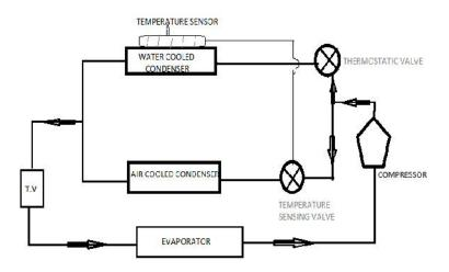
Figure 5: Heat Recovery in Domestic Refrigerator Using Two Condensers
