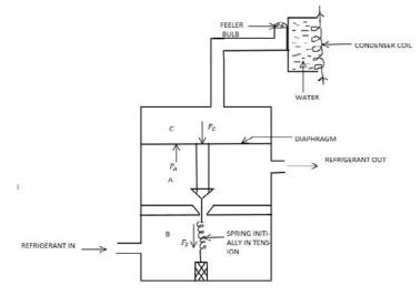
**Figure 3: Thermostatic Valve**
